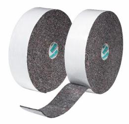
ASTORfilz 15720 Insulation felt for noise damping, i.e. to be used separation tape in dry wall applications. Also used for protection of window frames or other sensitive surfaces.
